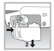
Access the light bulb by removing the cover as indicated in the diagram. Replace it with a similar light bulb within the power range indicated on the cover (max 10W).
